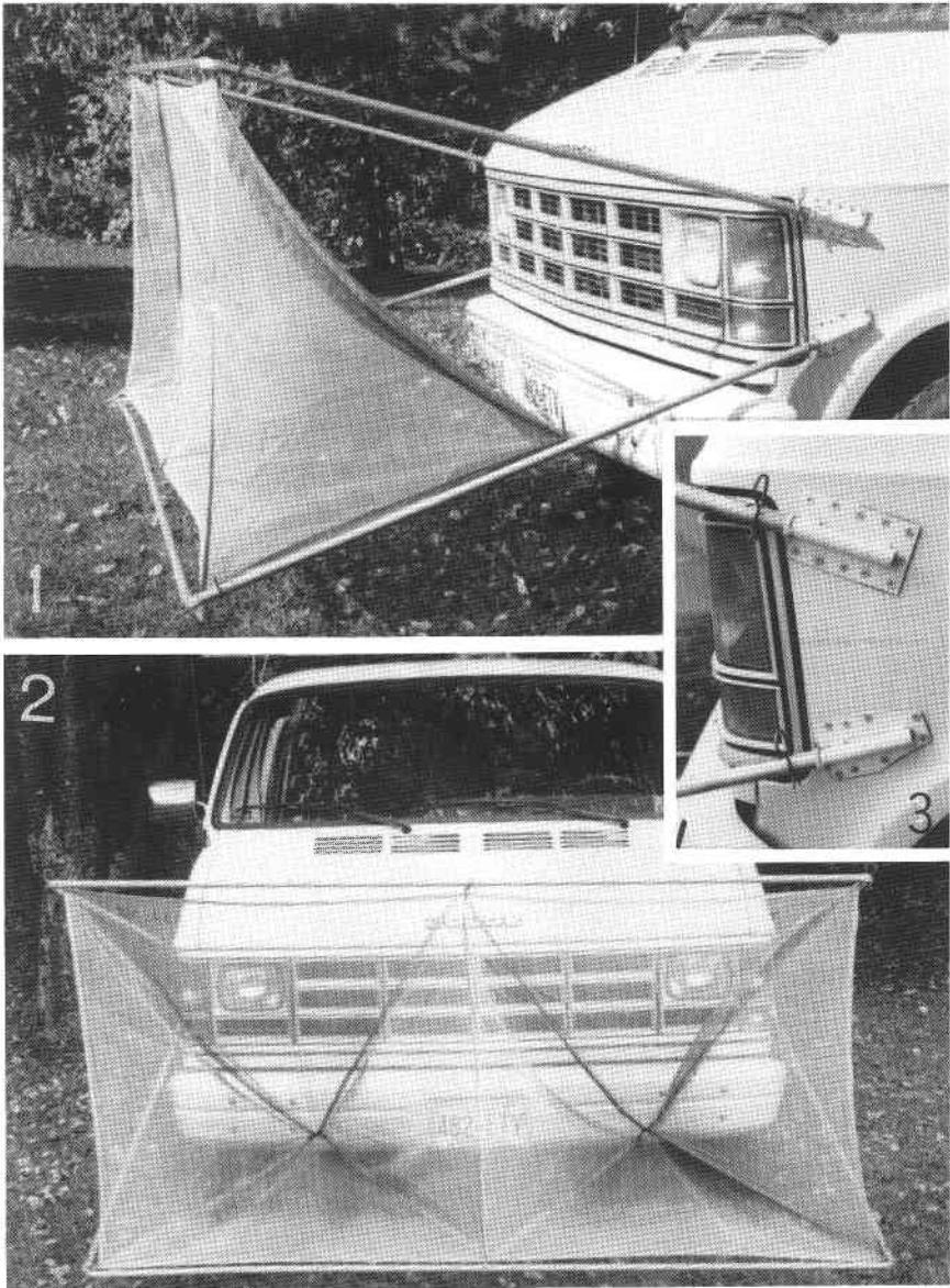
FIGS. 1–3. 1, side view of car-net assembly; 2, frontal view of car-net assembly; 3, inset to show permanently fixed side plates attached to vehicle, and hitch pin clips holding tubes onto interior prong from side plates.
